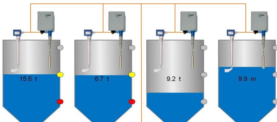
Full level status signal buzzer, tank wagon detection, shut off valve control, truck module
